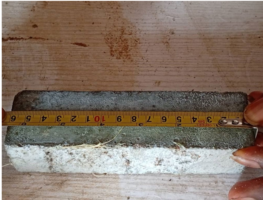
Fig. 5 Measuring length change after \text{MgSO}_4 exposure
