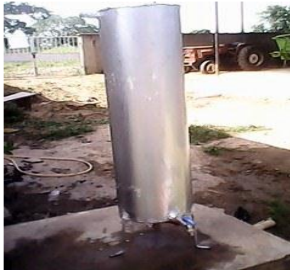
Figure 2: The slow sand filter for water purification
