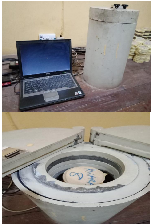
Fig 5: Experimental setup for sample radionuclides detection
