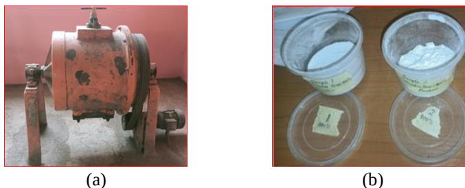
Figure 3. Ball milling process (a) and eggshell nanoparticles (b)
