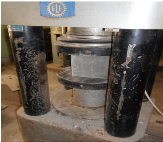
Plate 4: Compression testing of concrete cube
