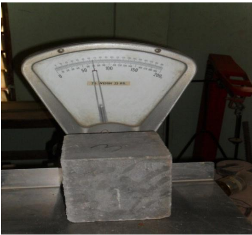
Plate 3: weighing of concrete cube
