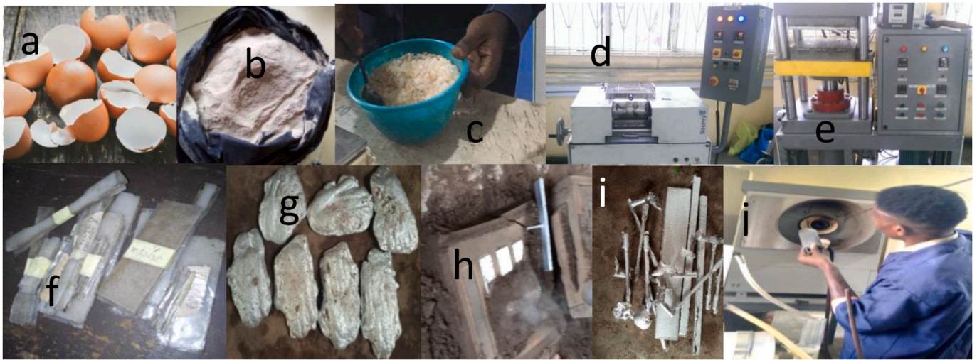
Fig. 1a. Pictures of materials and procedures for production of composites: (a) eggshells (b) date seed particles (c) mixture ready for pouring (d) roll mill extruder (e) hot compressive moulding machine (f) developed polymeric nanocomposite samples (g) Al-Cu-Mg lumps (h) broken sand mould to remove the as cast metallic nanocomposites (i) the as cast samples (j) putting samples inside the tube furnace for the heat treatment.
