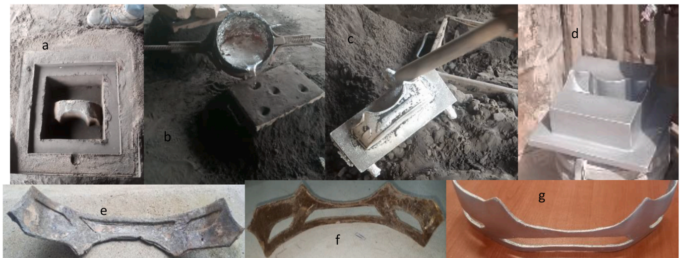
Fig. 12. Fabrication of bumper fascia prototype (a) mould pattern (b) pouring of metalli composite melt into the mould (c) As cast mould part [cope] (d) mould part (drag) (e) as formed bumper fascia prototype (f) trimmed bumper fascia prototype (g) painted bumper fascia prototype.
