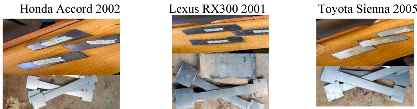
Fig. 2. Selected vehicles models serving as sources of bumper fascia for benchmarking the properties of the developed polymeric nanocomposites.
