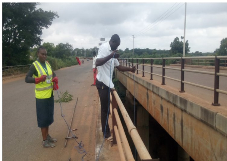
Fig. 2 Flow and scour depths determination at the Bridge location
