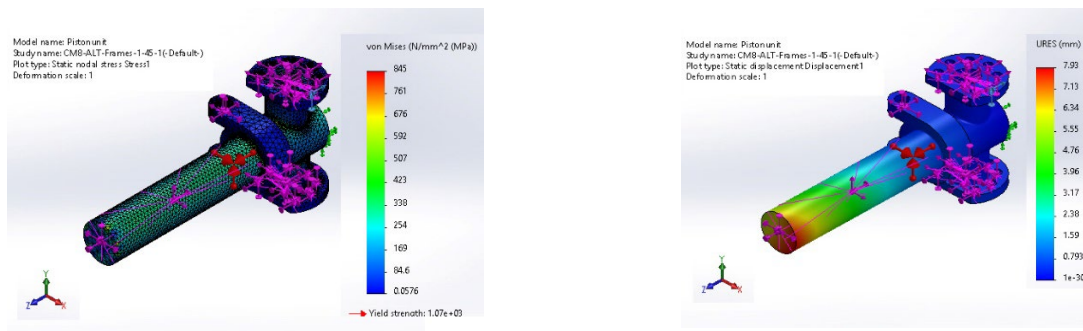
Fig. 12: Piston (Ti-6Al) (a) Stress analysis (b) Total displacement
