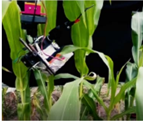
Figure 9.3 A robotic system for automatic in-field leaf disease detection [52].
