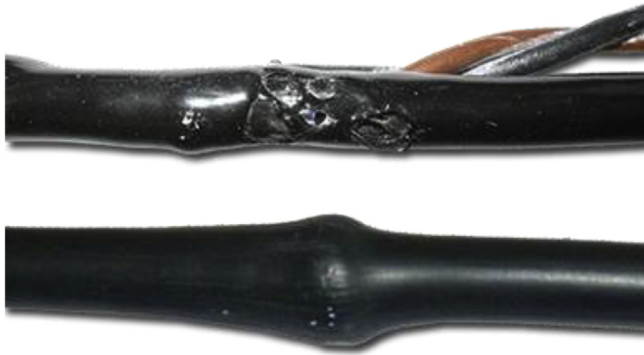
Figure 1. Electrical cable insulation with defects.
